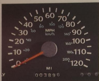
Figure 2.2 ▲ The speedometer for a North American car gives readings of instantaneous speed in both mi/h and km/h. Odometers for the U.S. market give readings in miles; those for the Canadian market give readings in kilometers.
